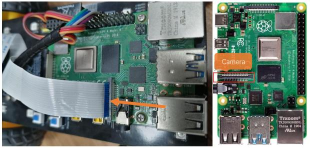
**The Blue side of cable should be toward to RPi USB port.** Connect another end of cable to raspberry pi. Please note front and back of the cable.
