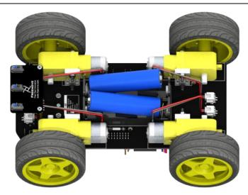
Finally, install two 18650 batteries. 2X 3.7V 18650 lithium **rechargeable** batteries without protection board. **It is easier to find proper battery on eBay than Amazon.** Don't assemble servos at present. The assembly about Pan Tilt will be introduced in next chapter. Just follow the tutorial step by step.
