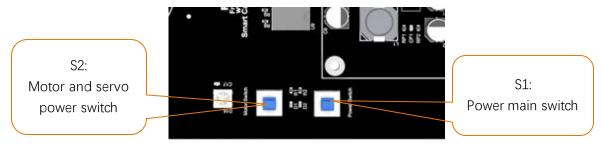
During the test, the motor will work. So you can disconnect the wheels or put it on the ground to avoid that it falls down and is damaged.Next, test RGB LED, motor, ultrasonic module, servo, etc.
