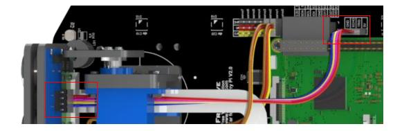
When connecting the ultrasonic module, you need **disconnect** the **Servo1** cable, so that the servo can be freely rotated, and after the wiring is completed, connect servo cable again. When wiring, you should keep the silk screen of the ultrasonic module and the smart car board consistent. Vcc should be is connected to 5V, Trig is connected to TRIG, Echo is connected to ECHO, and Gnd is connected to GND.
