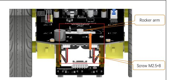
Keep the Rocker arm consistent with screen printing on smart car board. Use two screw M2.5\*8 to install it with smart car board.
