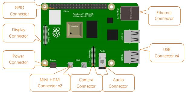
Hardware interface diagram of RPi 4B is shown below:
