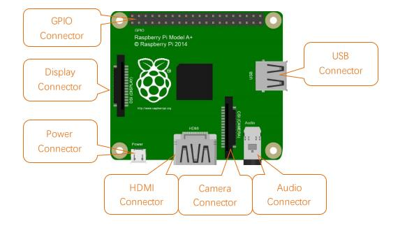
Hardware interface diagram of RPi 3A+/A+ is shown below:
