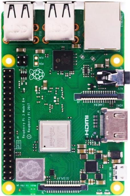
Model diagram of Raspberry Pi 3 Model B+:
