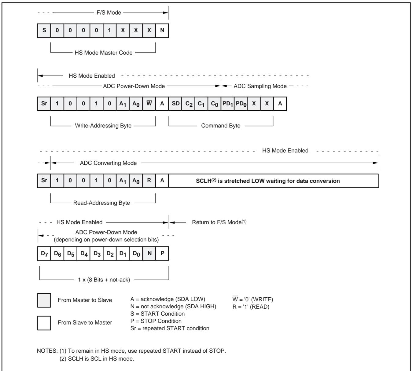
FIGURE 4. Typical Read Sequence in HS Mode.
