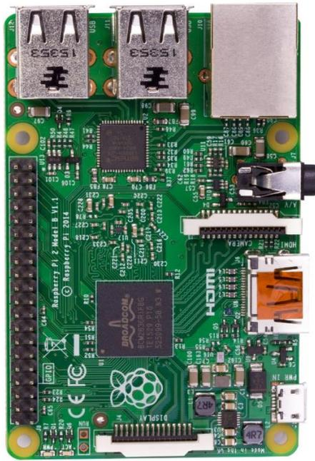
Model diagram of Raspberry Pi 2 Model B:
